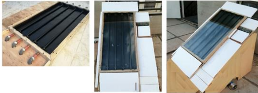
Fig. 3 - Solar collector installation
