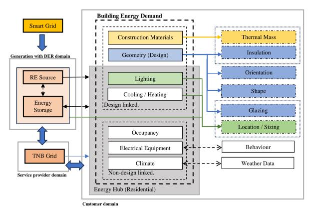
Fig. 5 - Proposed Design Optimization for Smart Grid (DOfSG) framework
