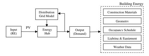
Fig. 4 - Optimization framework for distributed energy system ((Morvaj et al., 2016)
