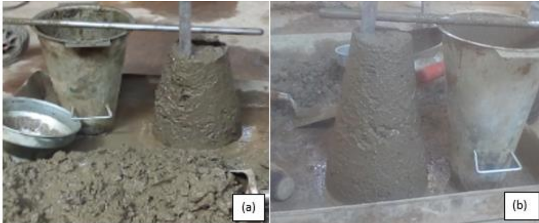
Fig. 5 - Workability of concrete with (a) 0% and; (b) 10% pumice content
