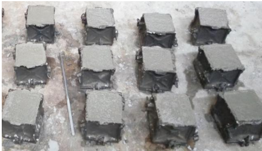
Fig. 4 - Photos of casted cube specimens
