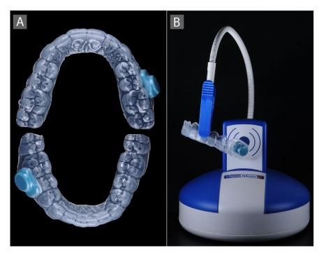
Figure 2- A- Upper and lower acetate trays with the microsensor attached to the buccal surface; B- Reading station for transferring data to the software
