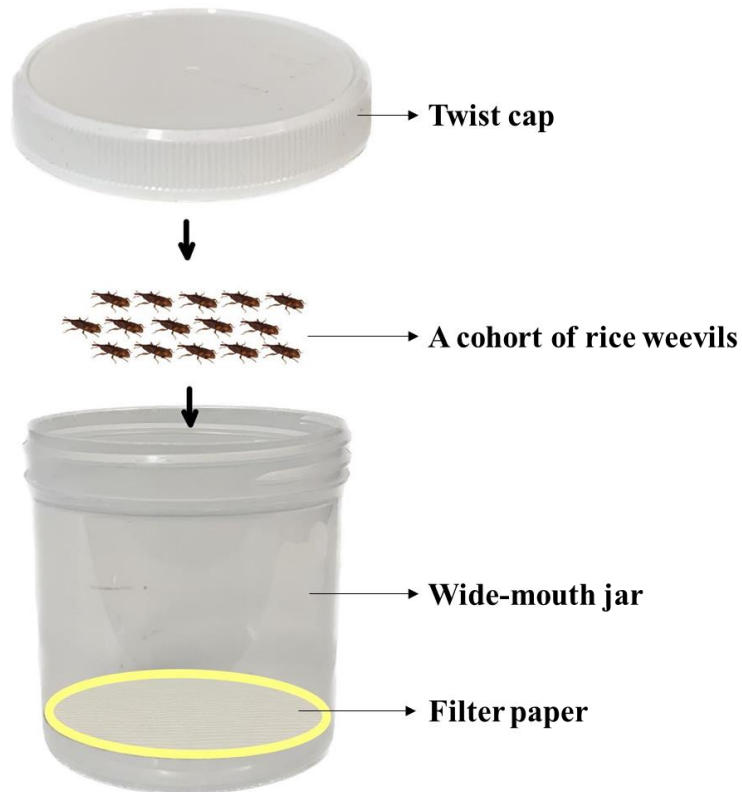
Figure 2. Design of Experimental container used in the study.
