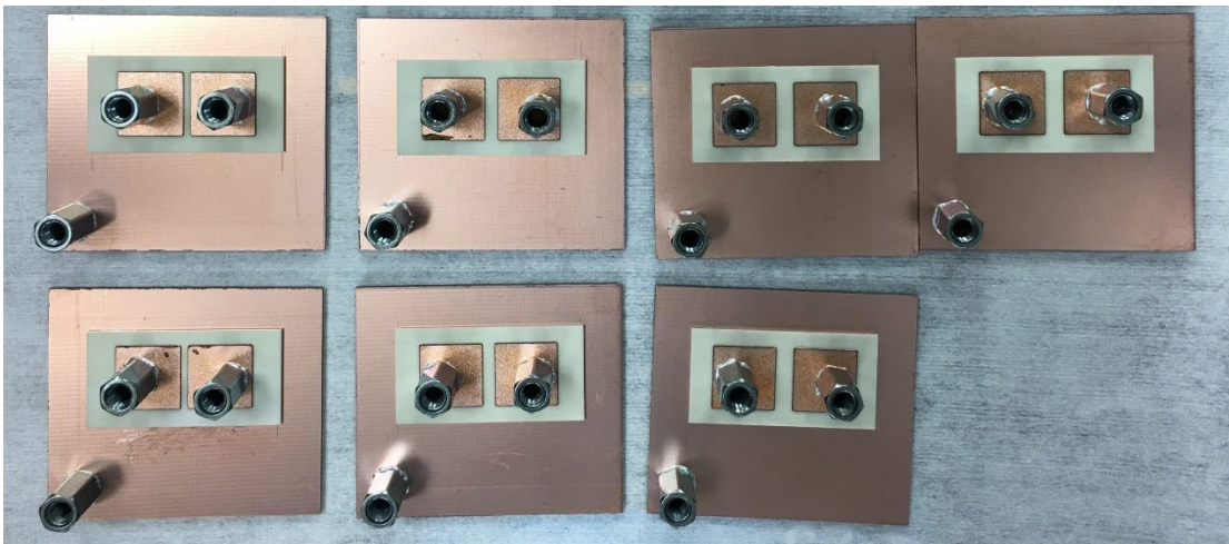
Figure 155. Terminals attached to DBC traces and FR4 base.
