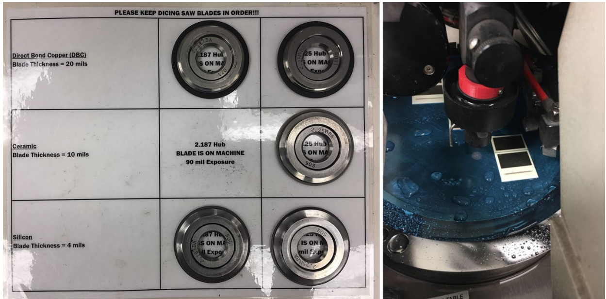
Figure 147. Dicing saw blades used for cutting various types of substrate materials (left) and ceramic substrate being diced by the appropriate blade in the dicing machine (right).
