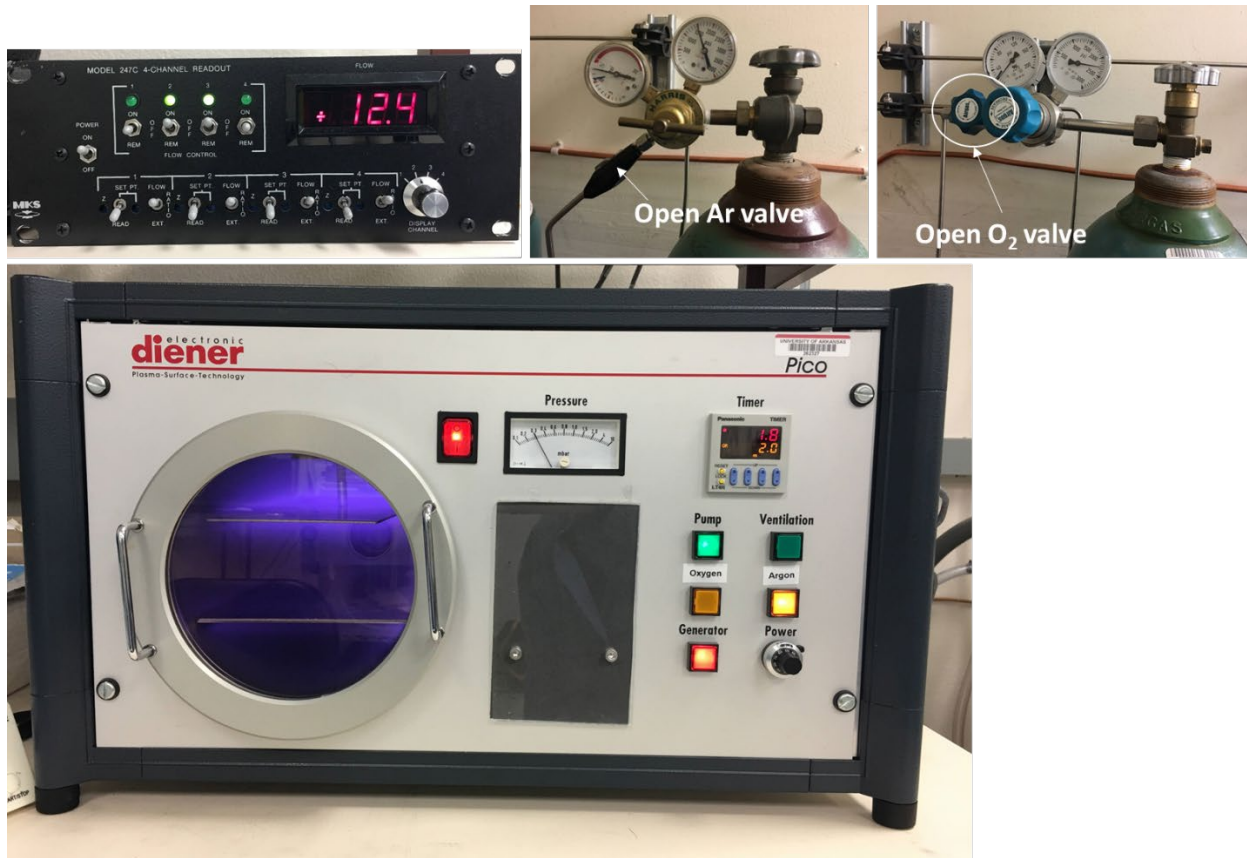
Figure 149. Diener electronic plasma cleaner (bottom) and its flow controller (top) and argon and nitrogen valves (right).
