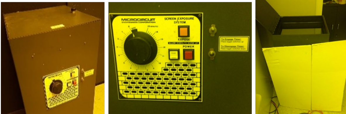
Figure 134. UV light exposure unit (left), its control panel (middle), and the top glass with lid open and whiteboard in front (right).
