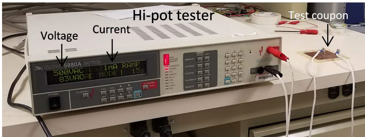
Figure 89. Test setup for AC voltage breakdown tests.
