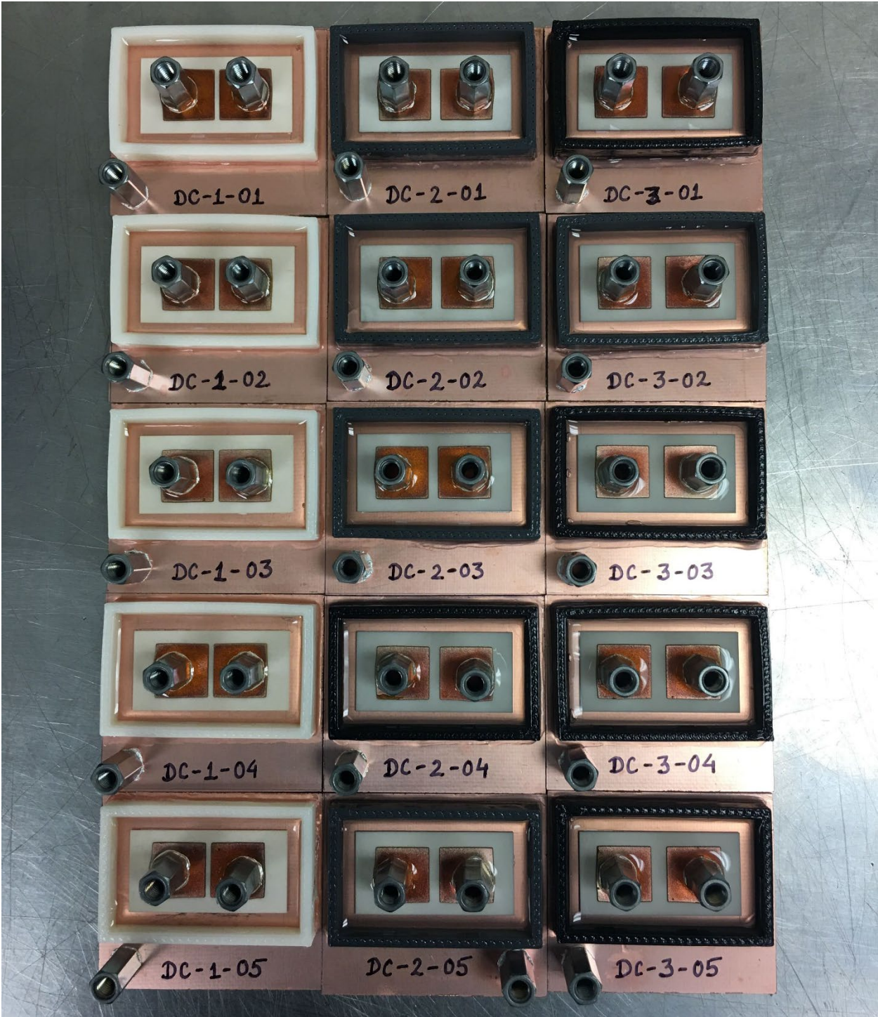
Figure 164. Samples after the dielectric gel curing process, and ready for testing.
