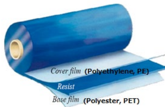
Figure 136. Dry film photoresist structure.
