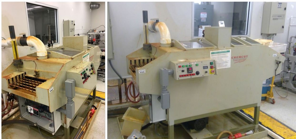
Figure 131. Chemcut Spray Etcher conveyor view (left) and control panel view (right).
