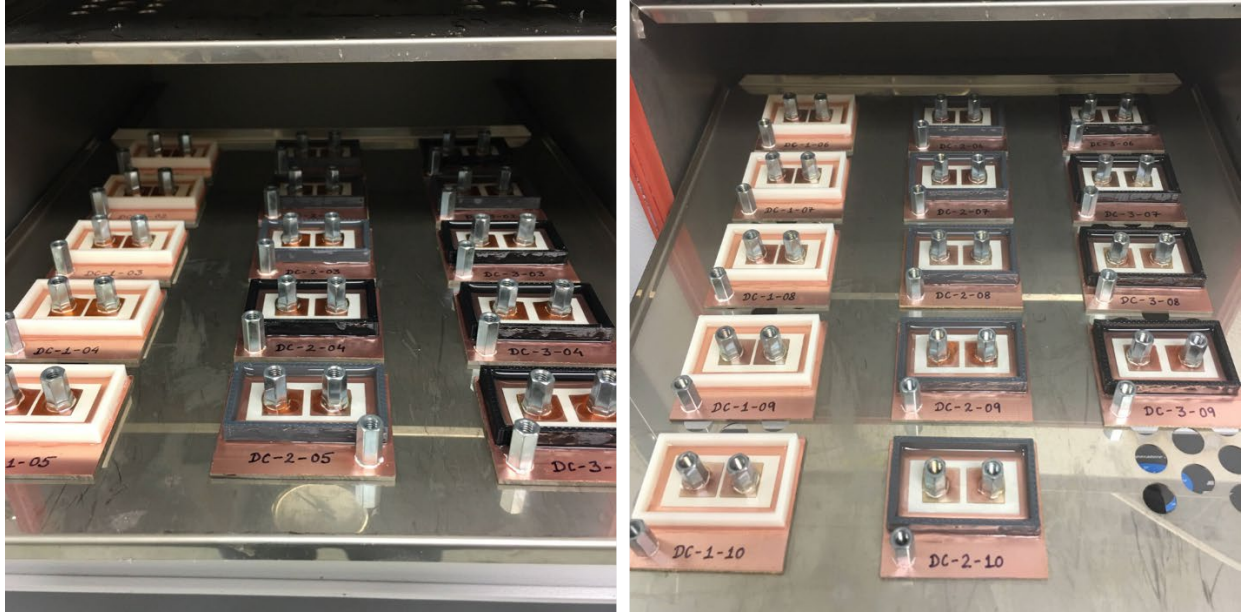
Figure 162. Samples on vacuum oven tray with gel within the 3D printed wells, ready to be vacuum cycled for bubble removal at room temperature.
