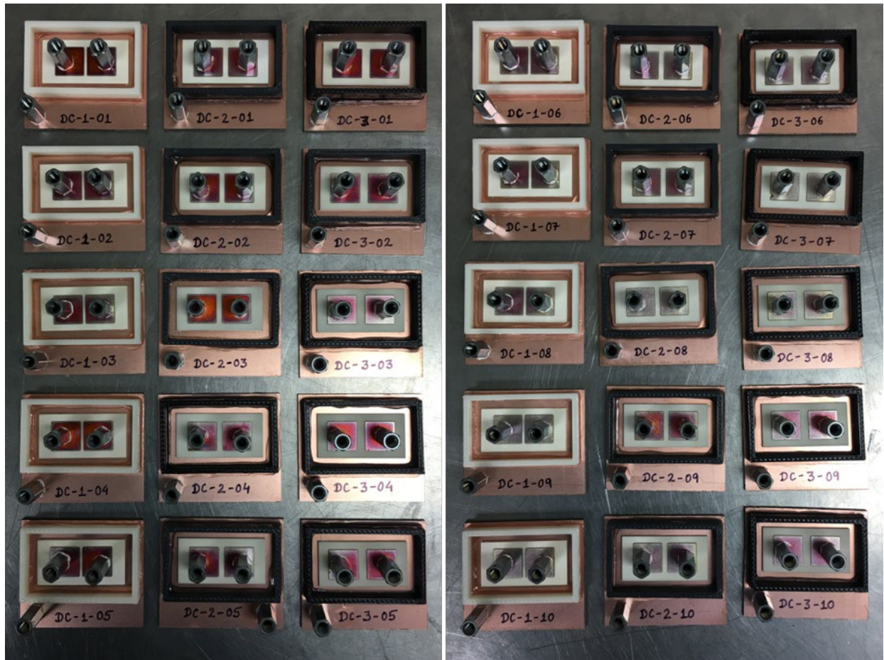
Figure 160. Housings attached on samples and glue cured over 24 hours.
