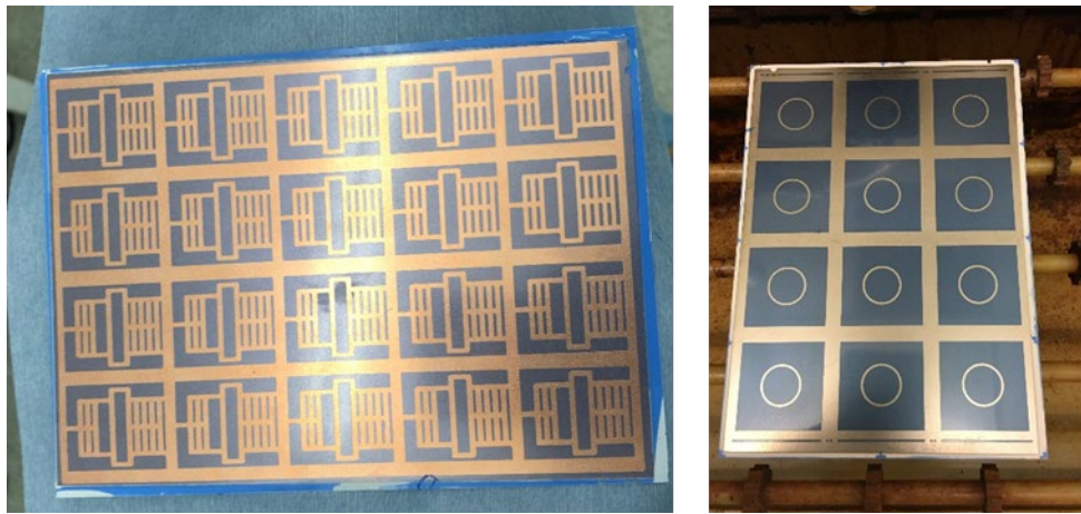
Figure 141. After development: all the blue film from the non-copper regions are rinsed away.
