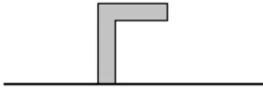
To find the center of mass of this simple object all that must be done is treat each side of the L shaped bar, as its own individual straight bar. The center of each bar will be the center of mass for each of our created pieces. The average between each of these point masses will be the center of mass for the total object:
