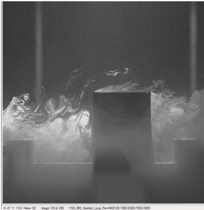
Figure 41 – Side view of a simulation of a chlorine release in the model with seed particles, used to determine the time interval between release and arrival at CONEX 11.4.
