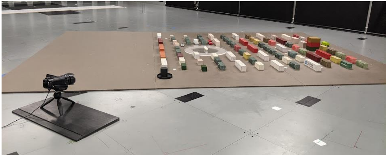
Figure 29 - Camera setup for flow visualization experiments in the MUE model, replicating Trial 5 from the JR-II field test.
