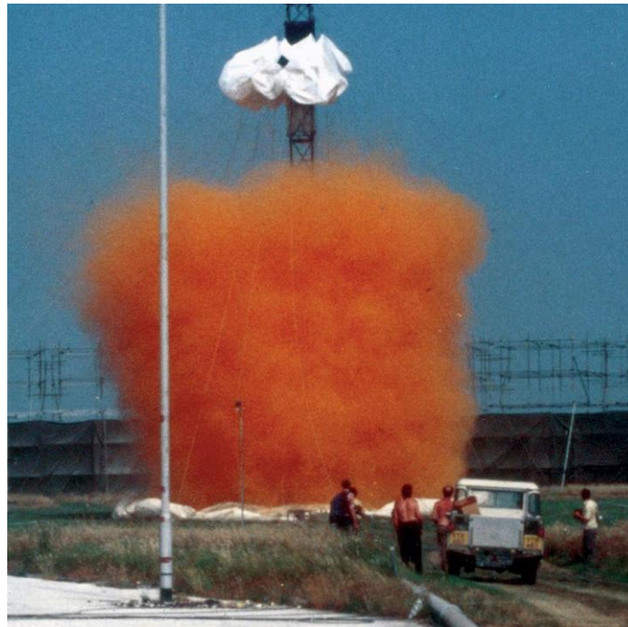
Figure 3 - Freon-12 release during the Heavy Gas Dispersion Trials – Phase II (Health & Safety Laboratory, 1985).
