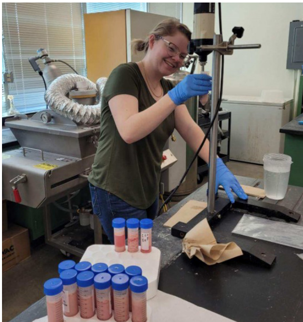
Jordan using the homogenizer to blend samples as a step in the thiobarbituric acid reactive substances assay.
