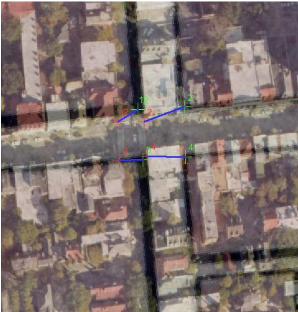
Figure 47: Zoomed-in image of the intersection of Broad Street and Church Street showing control point pair links on the overlay of the georeferenced “Clinton Map”.
