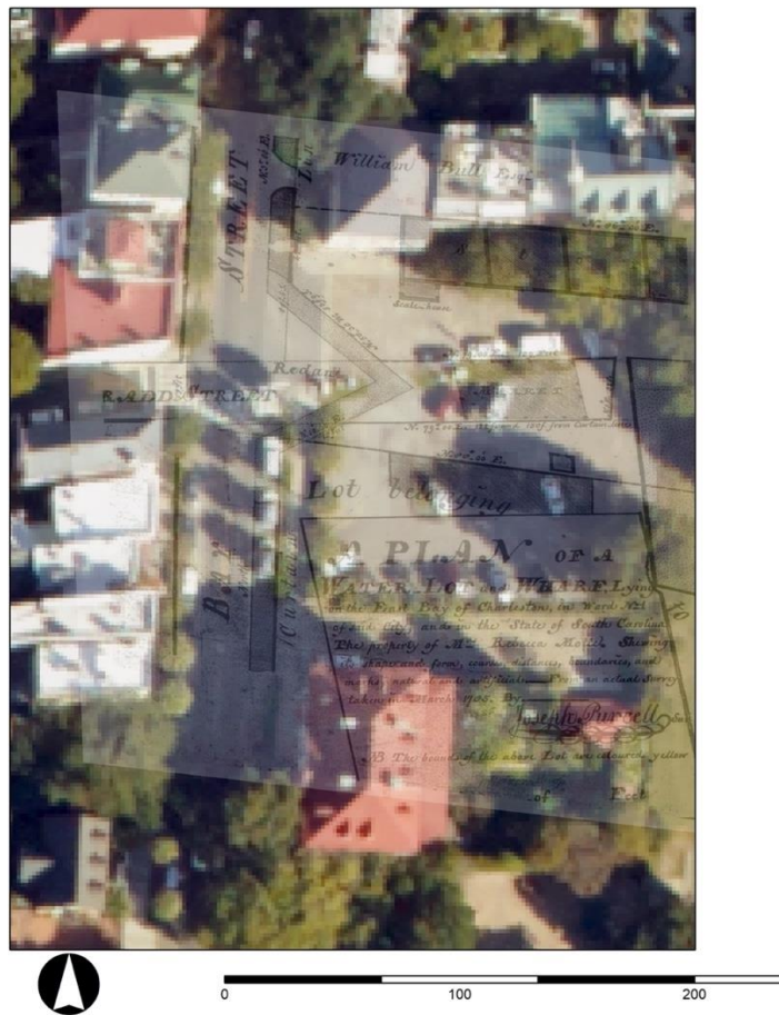
Figure 25: Georeferenced Tradd Street Redan Plat overlaid on the modern streetscape of downtown Charleston zoomed in to the intersection of East Bay Street and South Adger's Wharf.
