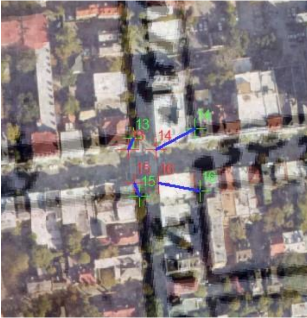
Figure 51: Zoomed-in image of the intersection of Broad Street and Church Street showing control point pair links on the overlay of the georeferenced Investiture of Charleston Map.
