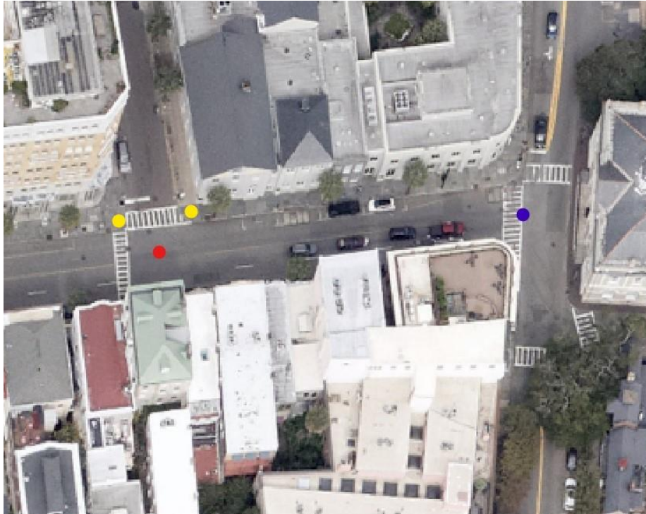
Figure 1: This map shows examples of control points: the red dot was taken at the center of intersections; the blue dot represents where a cross street runs into East Bay Street; and the yellow dots portray street corners.
