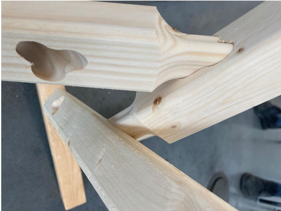
Figure 7. Robotically fabricated joints
