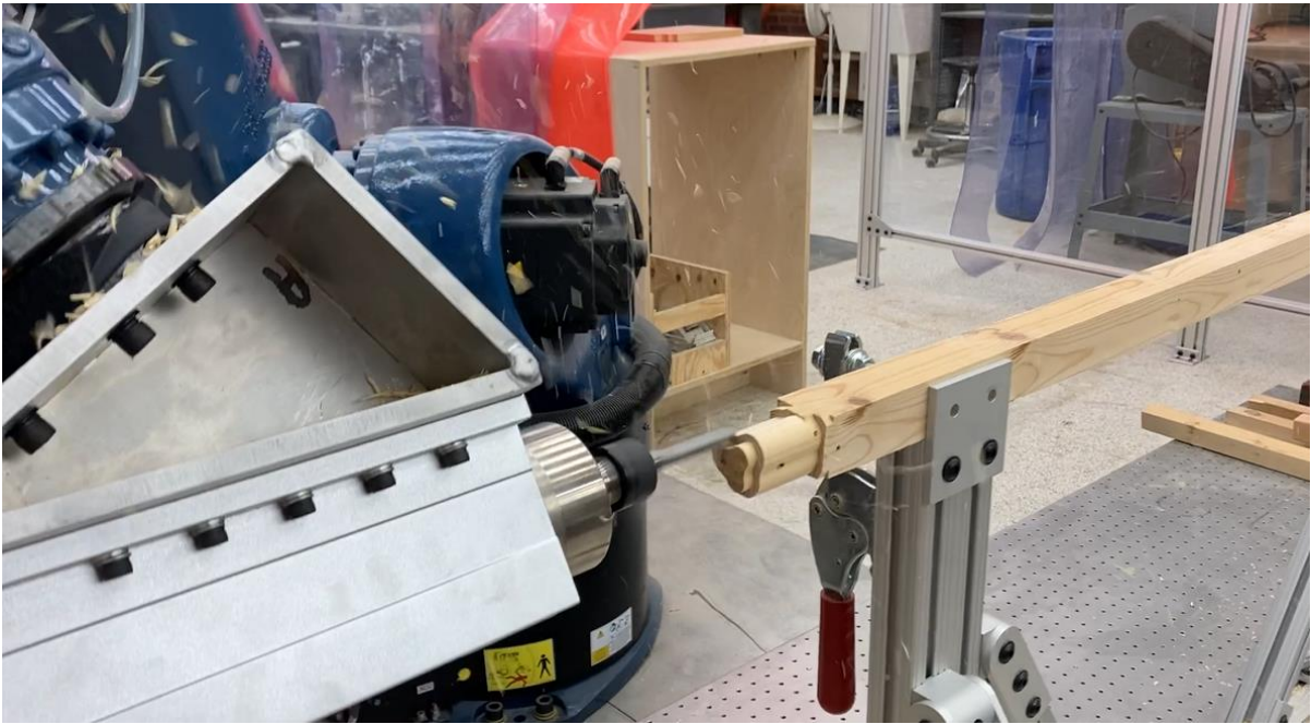
Figure D-11: Robotic fabrication of component-4
