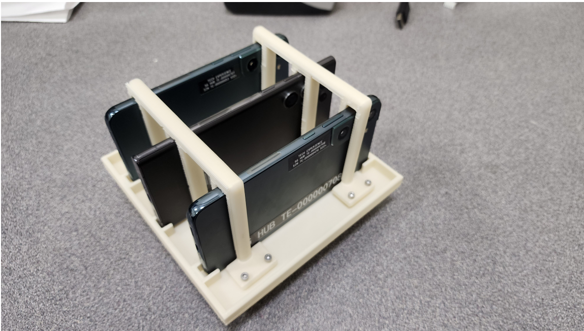
Figure 3.8: Three phones fitting in the 3D printed mount
