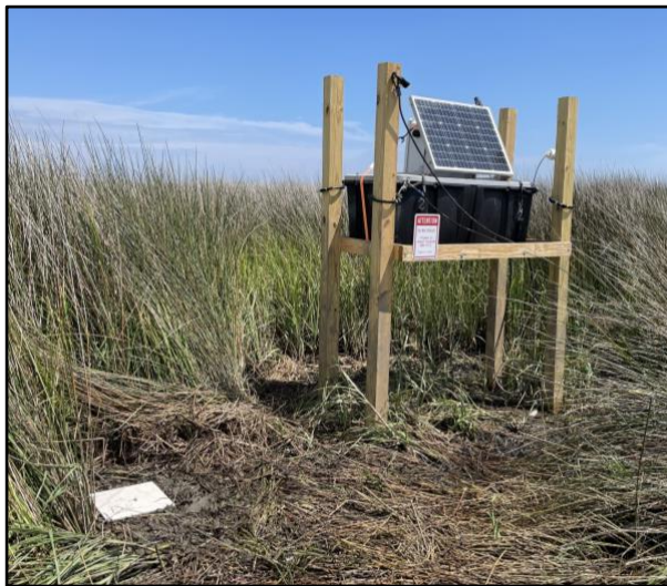
Figure 3.2. Conceptual design of the Net Sedimentation Tile (top) and infield photo of the Net Sedimentation tile deployed at TWC1 CO 2 gas flux monitoring station (bottom).
