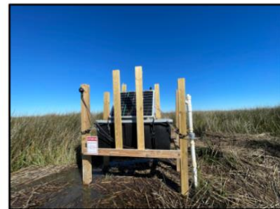
Figure 2.7. Hurricane Ian track map through NOAA's NI-WB NERR and CO 2 flux monitoring stations. Before and after Hurricane Ian images of TWC1 Monitoring Station, with the inclusion of supplementary posts to support rise and fall of the flotation power station.
