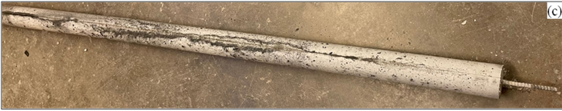
Figure 3.1. Small-scale precast drilled shaft (a) holder frame design, (b) constructed holder frame, and (c) final precast drilled shaft
