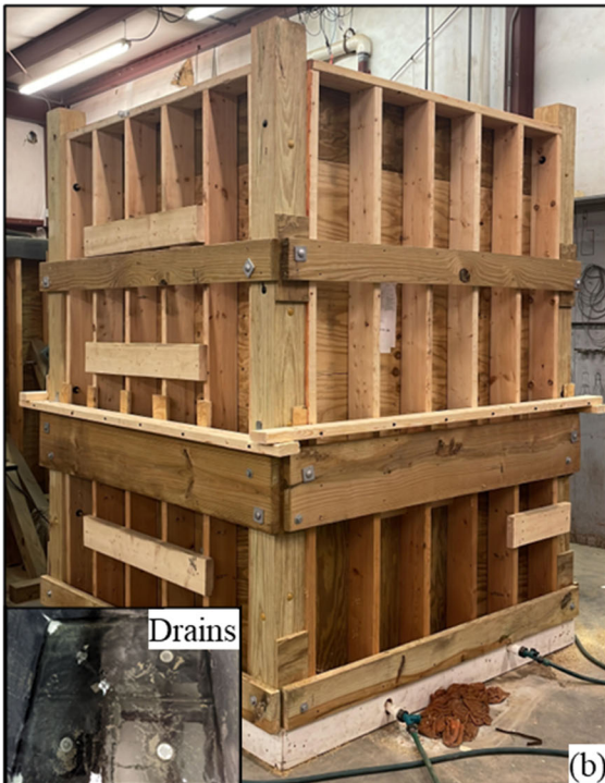
Figure 3.2. (a) Soil box drawing, (b) Constructed soil box, and (c) precast drilled shaft installed on the base layer
