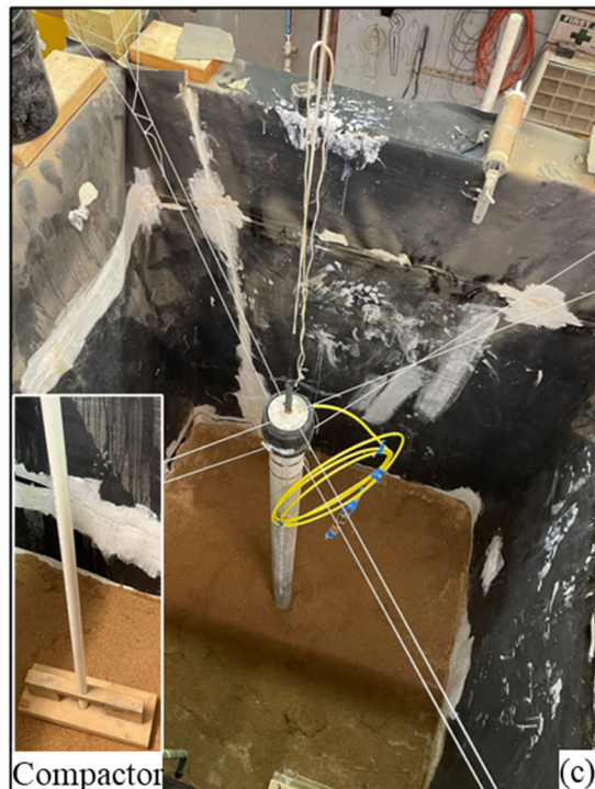
Figure 3.2. (a) Soil box drawing, (b) Constructed soil box, and (c) precast drilled shaft installed on the base layer
