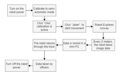
Figure 3. Flow Chart of Semi-automatic in Project-based Learning
