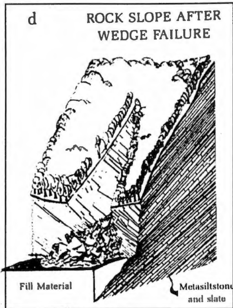
Figure 5.3: Wedge Failure. The valley portion of the site was likely created by this type of catastrophic event. Source: H. Moore (54)
