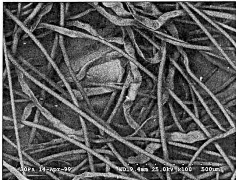
Figure 4.11 SEM Image Showing Disintegration of Bond (Intermediate Stage)
