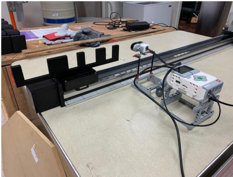
Figure 13. The black comb wall used for a supplementary portion of the infrared sensor experiment.
