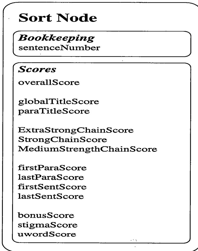
Figure 7.11: Internal Organization of SortNode.
