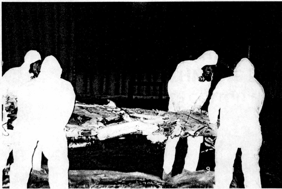
Figure B-19 Mishap Response Team in Full Personal Protective Equipment Moving Damaged Composite Wing Structure.
