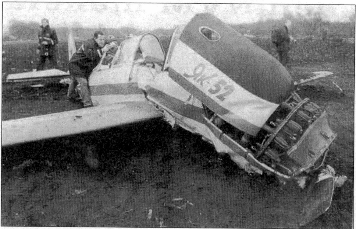
Figure 1-2 Fatal Yak-52 Accident Resulting From Inability To Recover From Flat Spin
