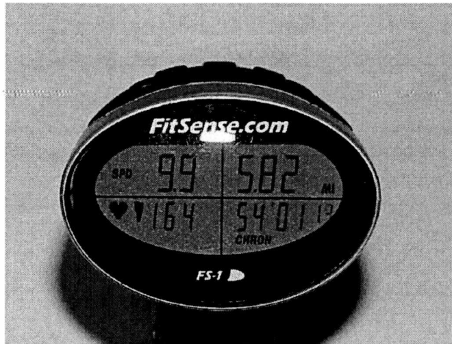
Figure 2 – The FitSense wristwatch receiver display. Top row: speed (miles · hr -1 ) and distance (miles); Bottom row: heart rate (beats · min -1 ) and total exercise time.
