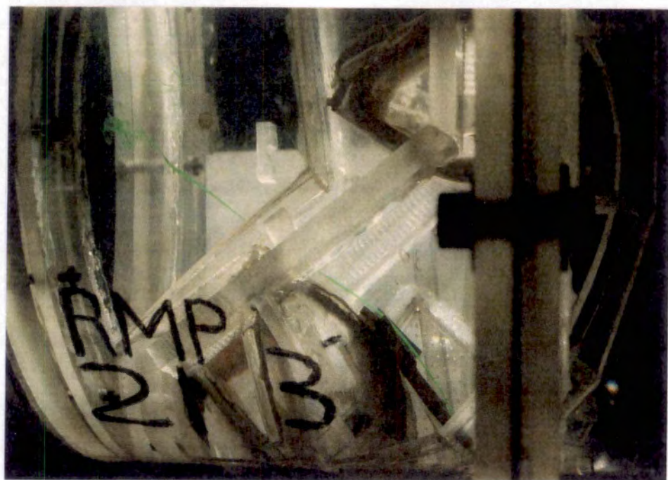
b. Zone 3, Ramp Displaced Toward Sidewall
