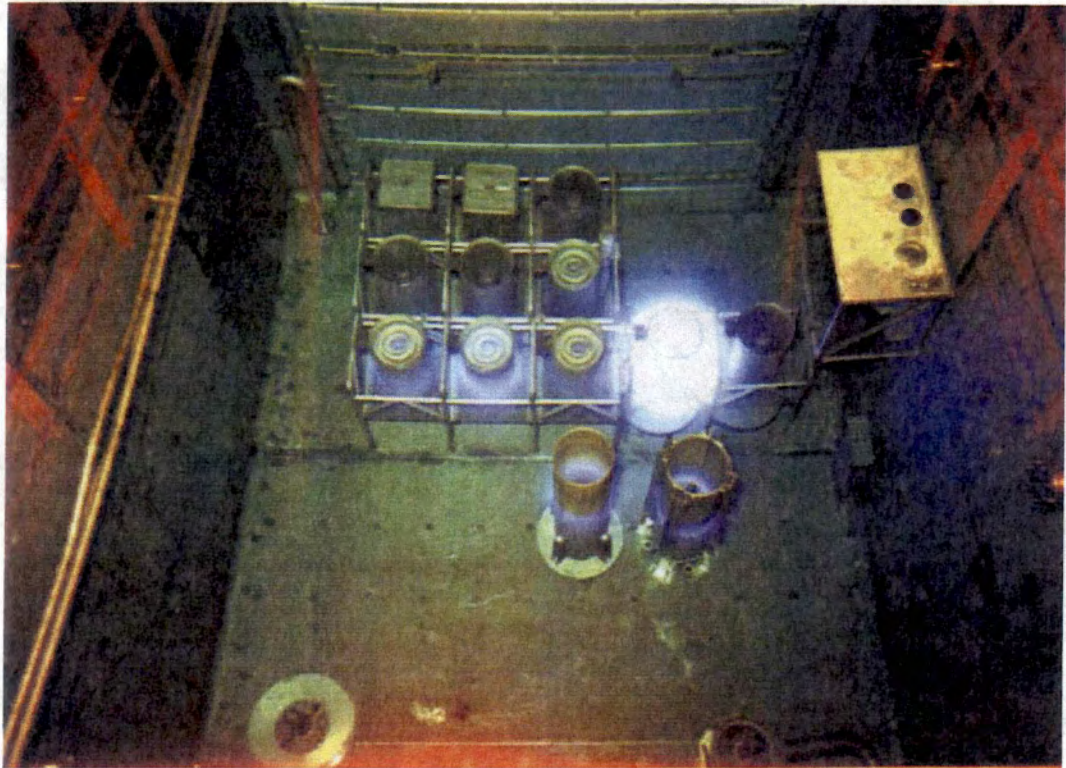
Fig. 3.7. SNF elements in the HFIR SNF pool.
