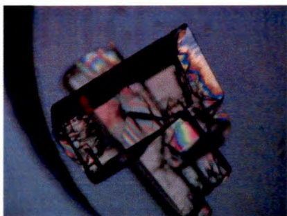
Figure 3.7: A very large nucleosome core particle crystal grown in a DCAM aboard the Mir space station.
