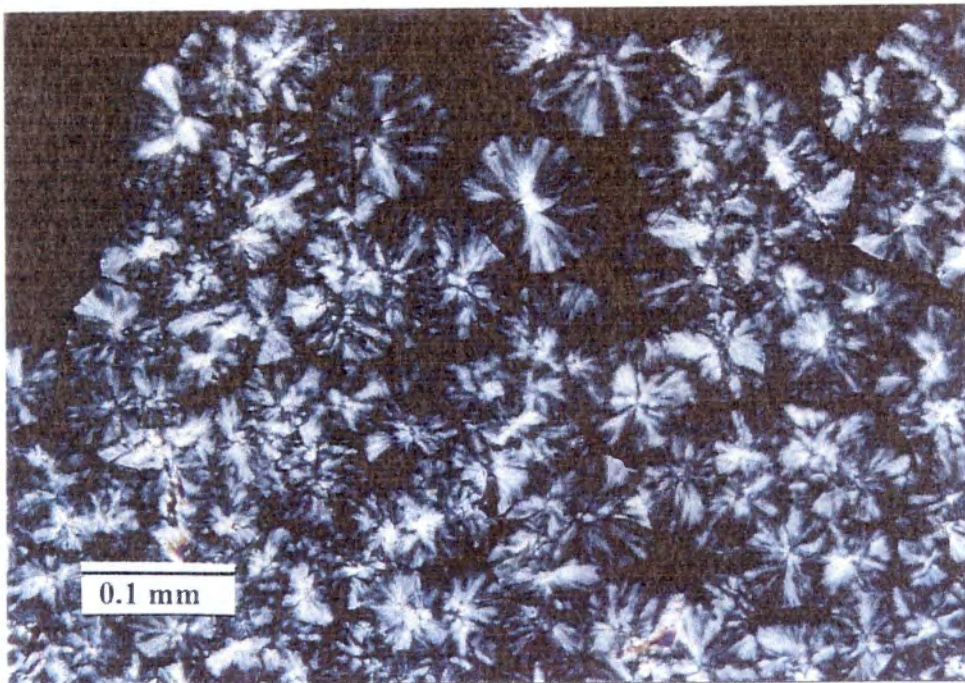
Figure 52: Photograph of spherulites from the X3 specimen (20X).
