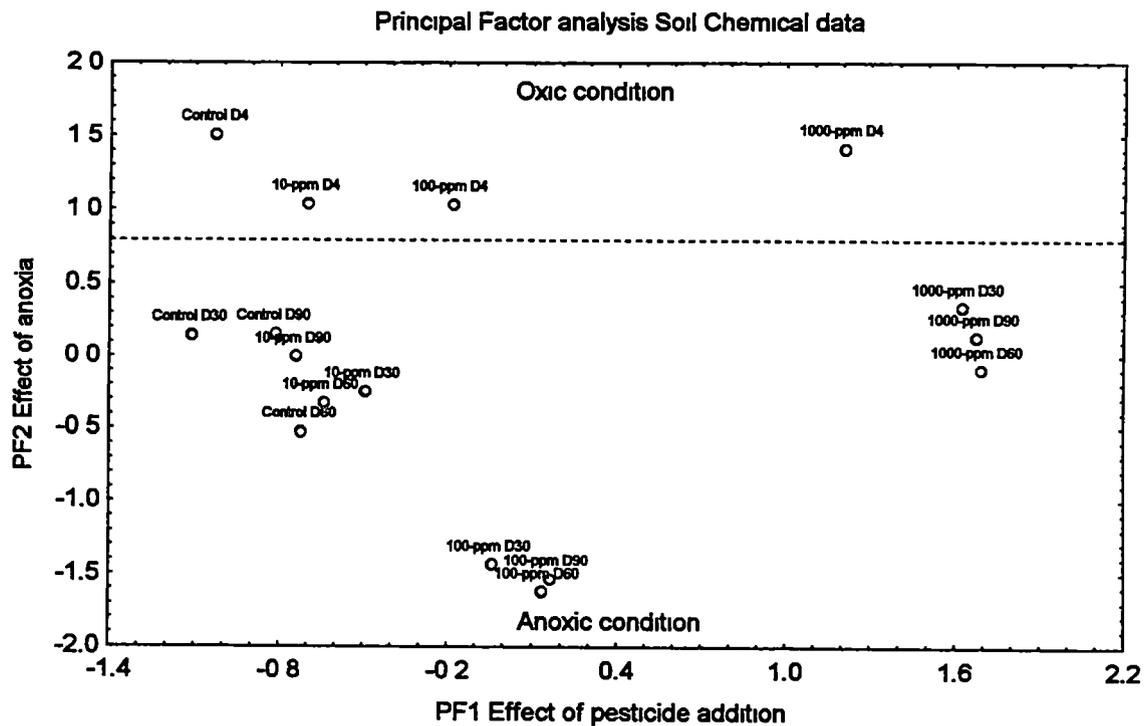
Figure 2-10. Factor analysis of soil chemical data. The variance explained by the two rotated factors are 28 and 24% respectively, with  $n=4$  for each point. This graph illustrates the effect of pesticide addition and increasingly anoxic conditions in the system.
