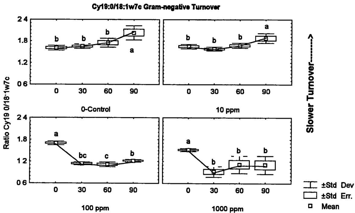
Figure 3-11. Cyclopropyl19:0/18:1w7c ratio over time, an index of Gram-negative turnover. N=4 and x-axis is days. Within box same letters are not significantly different according to LSD ( $\alpha=0.05$ ).
