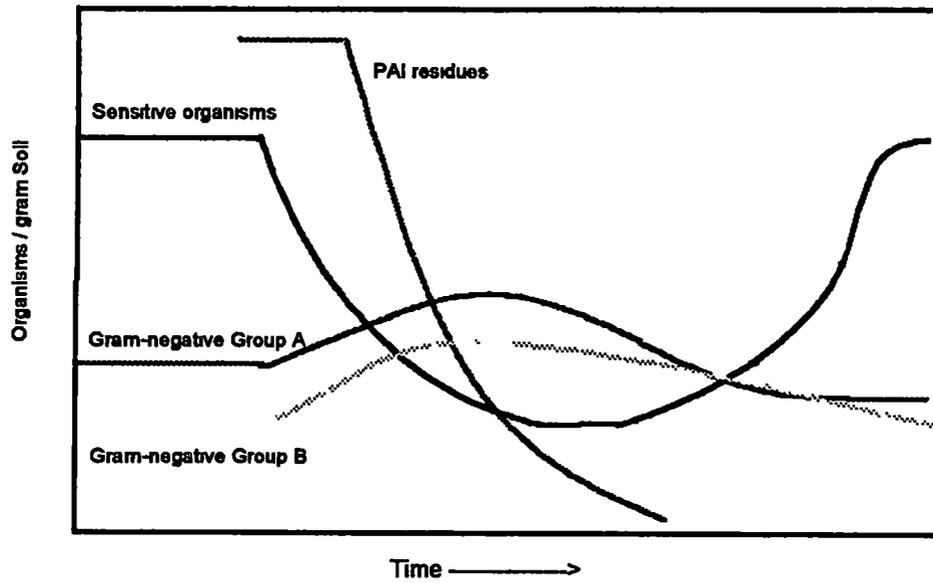
Figure 3-16 Soil microbial response model over time of Gram-negative group A and B organisms at 100-ppm. Both sub-populations are able to increase relative percentage and biomass.
