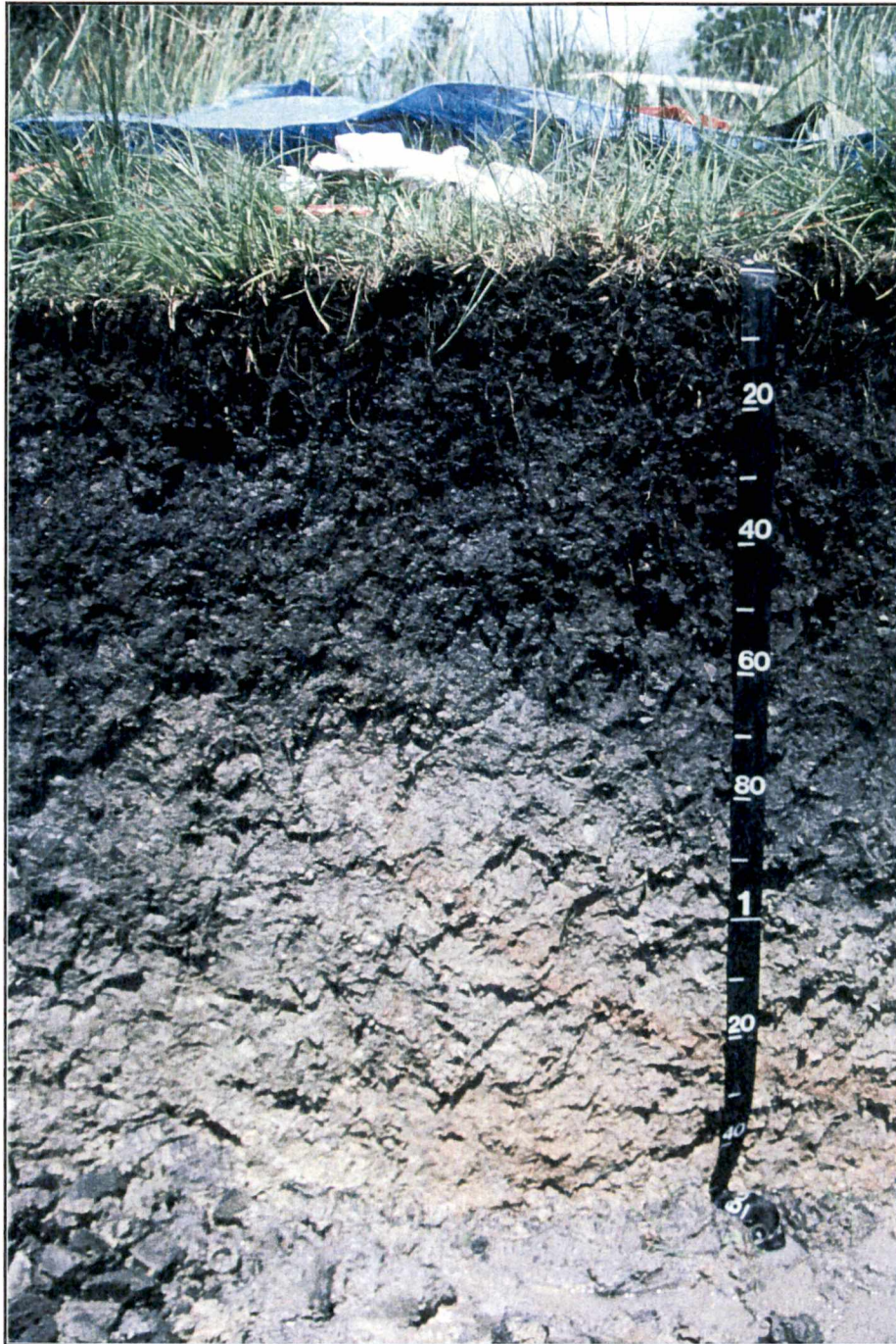
Figure 3. Field shot of Lake Charles microhigh pedon from Harris Co. (Armond Bayou), Texas shows a depth of ~ 1.5m. Slickenside faces are observed concentrating more toward the bottom of the profile and along the edges of the microhigh.
