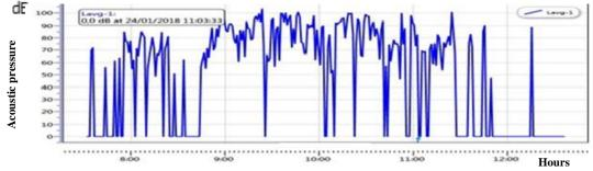
Figure 4- Graphic illustration of continuous noise levels emitted by the chainsaw.
