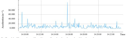
Figure 2- Graphic illustration of hand/arm vibration levels emitted by the pole saw.
