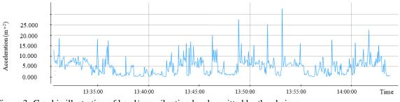
Figure 3- Graphic illustration of hand/arm vibration levels emitted by the chainsaw.
