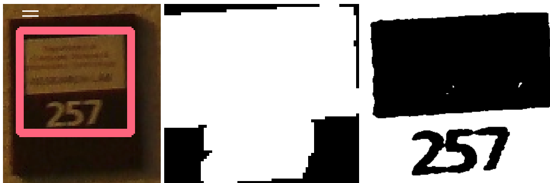
Figure 32: Due to the lighter foreground areas blobbing together in more dilation iterations, the whole area is picked
