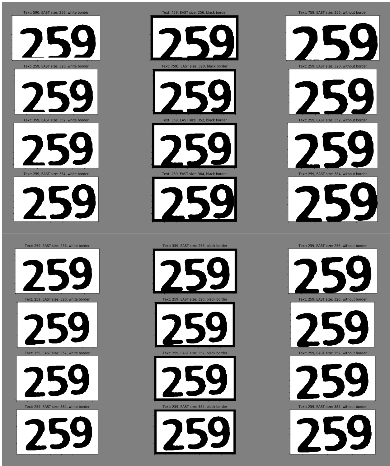
Figure 42: EAST text region crops with white border, black border, no border. Above is no buffer, bottom is 15 pixel buffer. Text reading improves when more image is selected.
