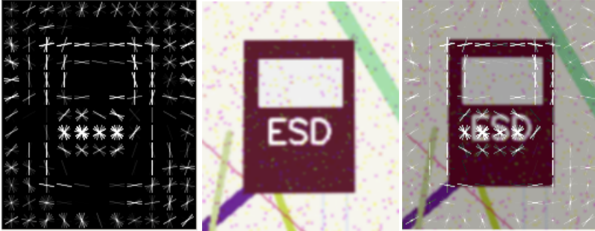
Figure 16: HOG created with a specifically-generated dataset
