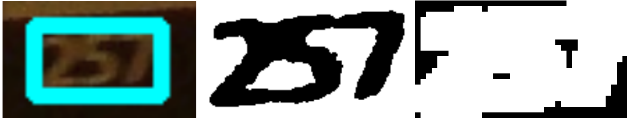
Figure 33: Less dilation iterations gives better separation
