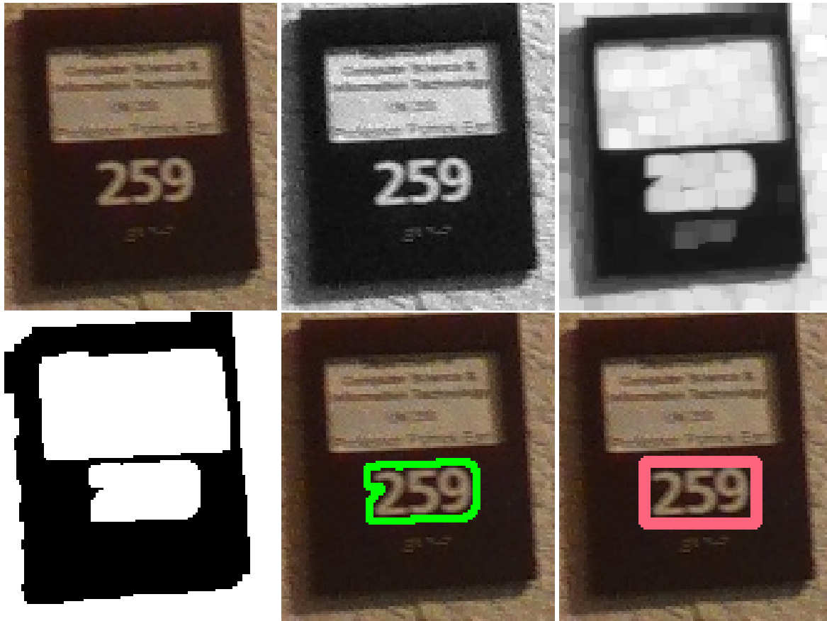
Figure 28: Image, grayscale, dilated, thresholded, contour, bounding rectangle progression
