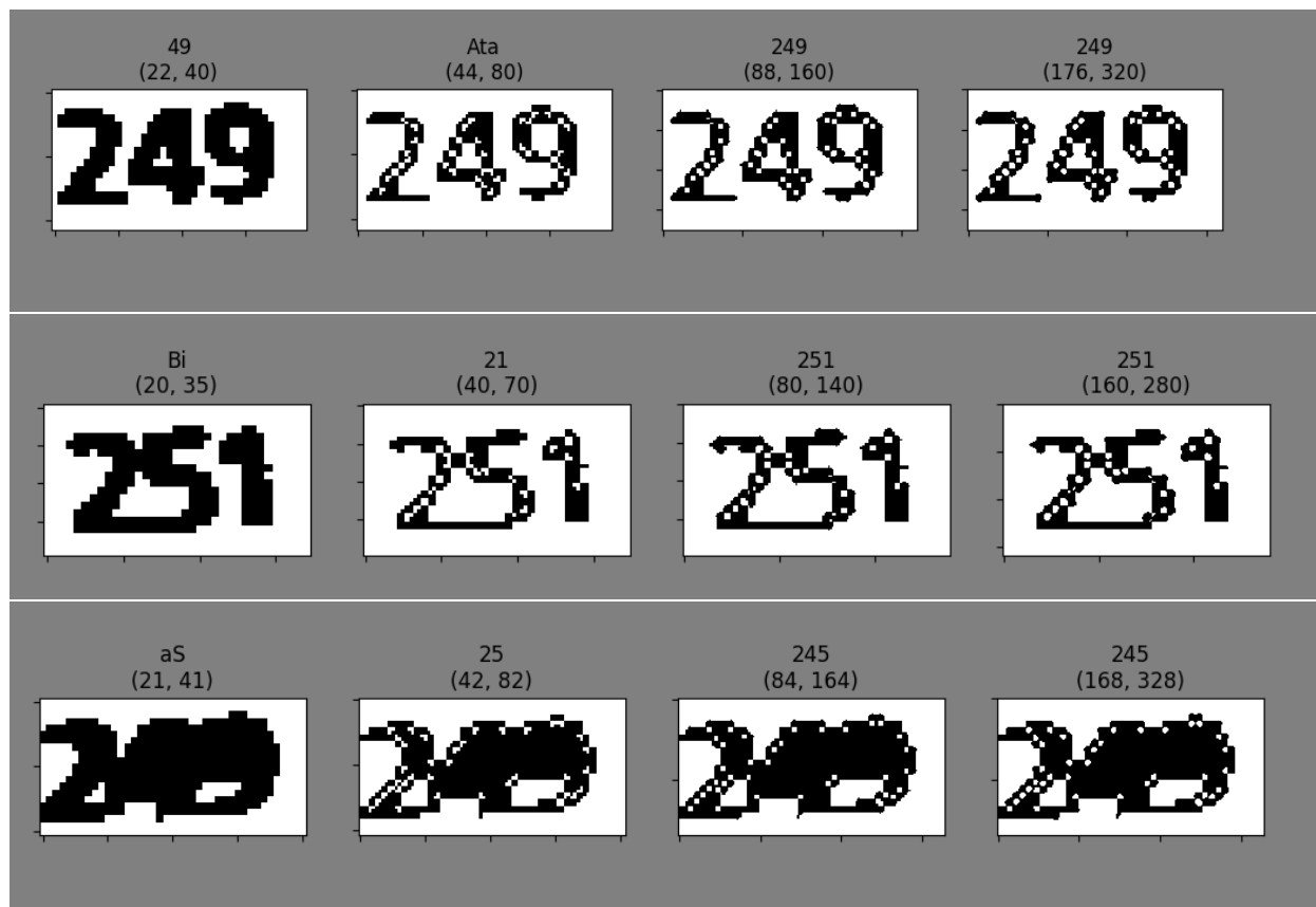
Figure 40: Resizing after thresholding the image. larger seems to be better, but the image quality is quite poor and text is misread
