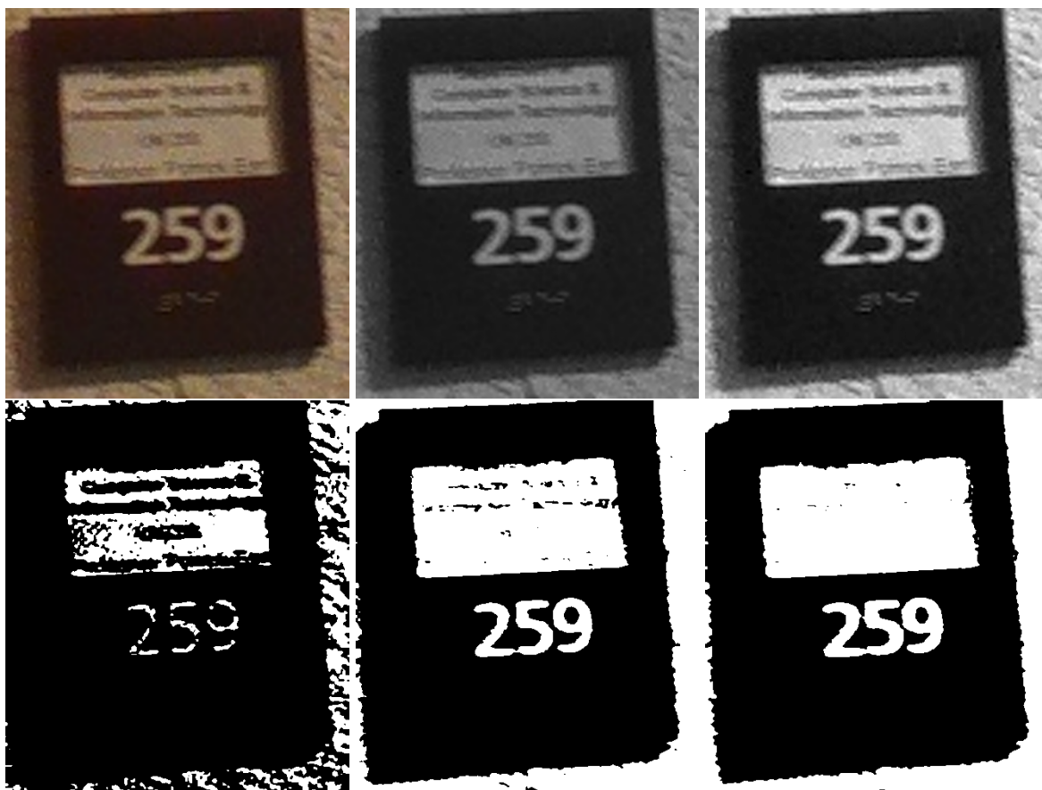
Figure 25: Plain image, converted to grayscale, and with the rescale_intensity . The results below are both thresholded with the same value range (125), but the image in the middle is the result of the rescaled intensity. The bottom image on the right is the result of using Otsu's thresholding on the grayscale image. Note the similarity to the rescaled image.
