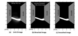
Figure 2. Image Processing a) Original 8 bit image, (b) converted binary image (c) post processed image
