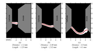
Figure 3. Arc length calculation at different gap distances a) at 1.2 mm, b) at 2.4 mm and (c) at 2.8 mm.
