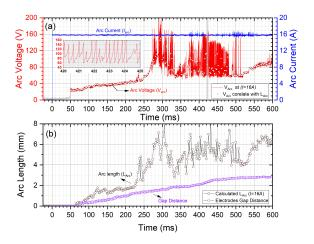
Figure 5. Voltage waveform at 16 A during contact switching process, (b) measured arc length for 16A
