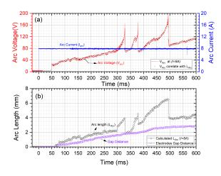
Figure 4. Voltage waveform at 8A during contact switching process (b) Measured arc length for 8A
