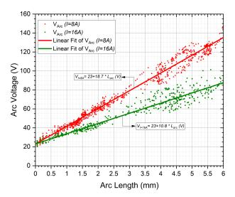
Figure 6. Voltage over the arc length plot for 8 A and 16 A for each three experiments along with the linear regression analysis
