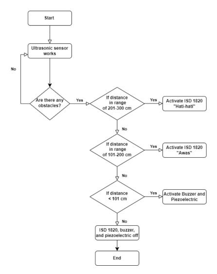
Figure 2. System flow diagram
