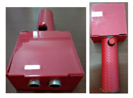
Figure 4. Smart cane prototype
