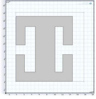
Fig.2 Structure of the metamaterial.
