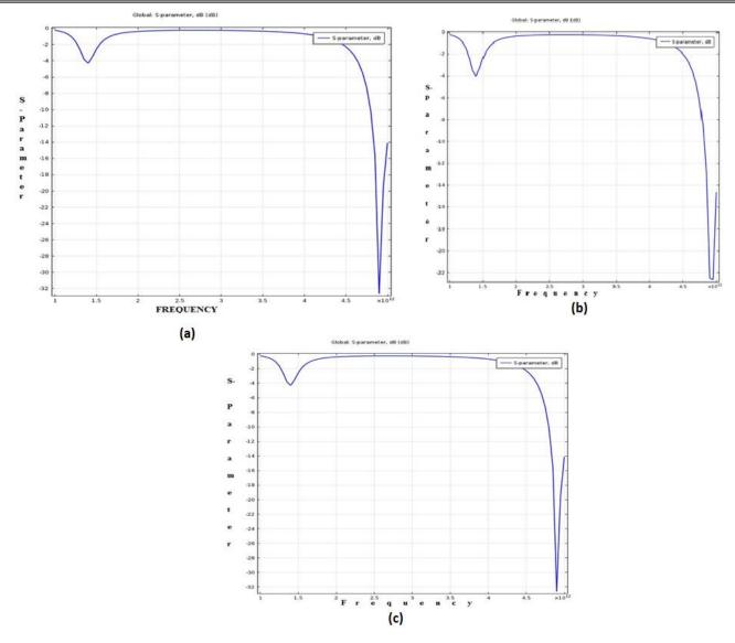
Fig. 5 Reflection coefficient: (a)with Gold, (b) With Silver, (c)with Copper
