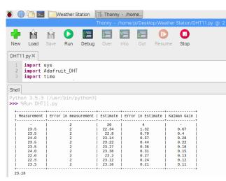
Fig.2: Reduction of error after applying Kalman filtering
