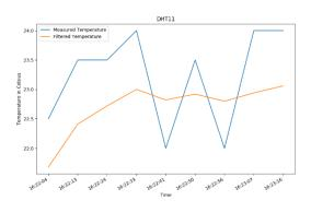
Fig.3: Comparison of temperature readings after applying Kalman filtering
