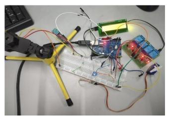
Fig 9: Top view of the home automation system showing differen sensors and modules
