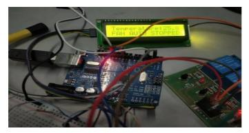
Fig 10: Temperature is less than the threshold and the ystem switching Off the fan
