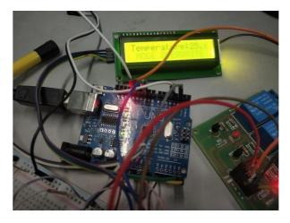
Fig 12: Overwrite mode of the Home Automation System. Once all the mode and conditions are tested successfully for the Home Automation System, the whole setup is now assembled inside a plastic cabinet. The assembled system is shown in fig 13. The sensors like DHT 11 and PIR are mounted on the outside of the assembly to make it easier to monitor the movement and temperature respectively.
