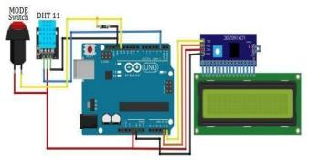
Fig 6: I2C module, LCD, DHT 11 and Arduinoconnection
