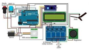
Fig 7: Complete wire diagram of the HomeAutomation System D10 of the Arduino is connected to a servo motor. The Vcc and GND terminal of the servo is connected to the 5V and GND of the system. The arduino code is generating a PWM signal which is send to the servo through the D10 pin of the Arduino. The PWM signal controls the rotation of the servo.
