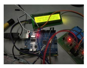
Fig8: Home automation system with all the components connected
