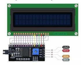
Fig 5: I2C module, LCD and Arduino connection
