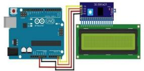
Fig 4: I2C module and LCDconnection
