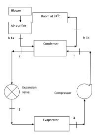
Fig. 1. VCR schematic with R134a as refrigerant for office room to be maintained at  $24^{0}C$  for January
