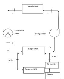
Fig. 2. VCR schematic with R134a as refrigerant for an office room to be maintained at  $18^{\circ}$ C for May
