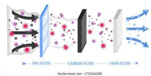
Fig.5. Schematic layout of air filter.[3']
