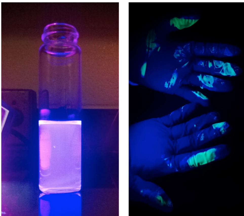
Figure 3. The observed fluorescence in the synthesis of Bisbenzothiophene (BBT). The image on the left displays BBT dissolved in acetone. This was apparent at 365nm (a long wavelength). The right picture exhibits the fluorescence of BBT that arose after the addition of acetic anhydride. This was captured at 254nm (a short wavelength). Fluorescence demonstrates the ability of the molecule to absorb and reemit light. These fluorescent molecules have applications in biological fluorescent probes and tags. 3
