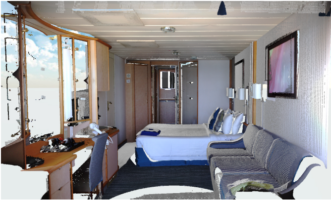
Fig. 2. Scanned Point Cloud
