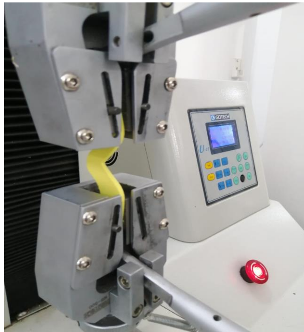
Figure 7: Universal Testing Machine Used in the Study with Sample
