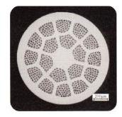
Figure 2.14: BSCCO Multi-Filamentary Wire [72]
