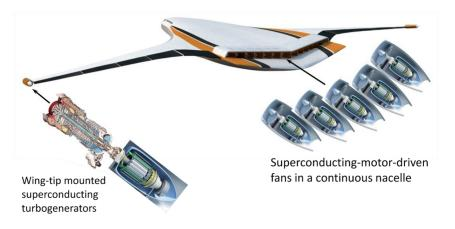
Figure 1.5: NASA N3-X Aircraft Concept [23]
