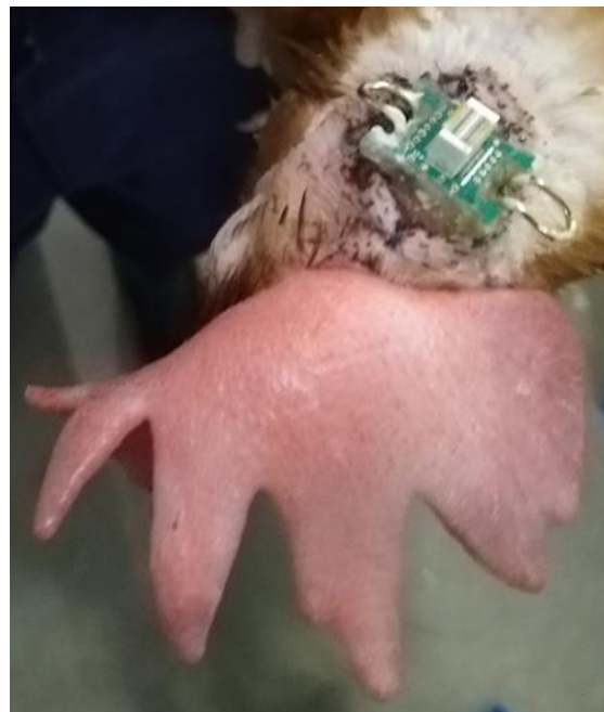
Figure 1. Implanted electronic interface board (EIB) microchip with metal hooks on either side to secure the logging device with rubber bands.
