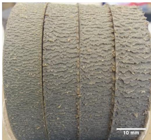
Figure Error! Main Document Only.. The fully developed abrasion pattern under 8 N, 12 N, 16 N and 20 N normal force from left to right for NR0.
