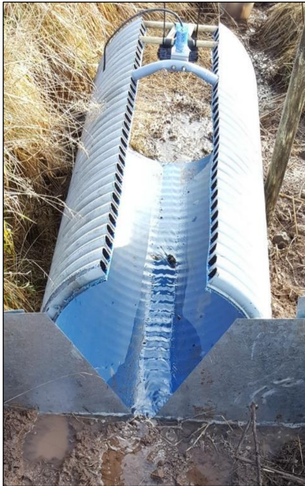
Figure 3.11: Photograph demonstrating experimental set up of Plot 5 with “V notch”; photography has been taken by the author looking downslope
