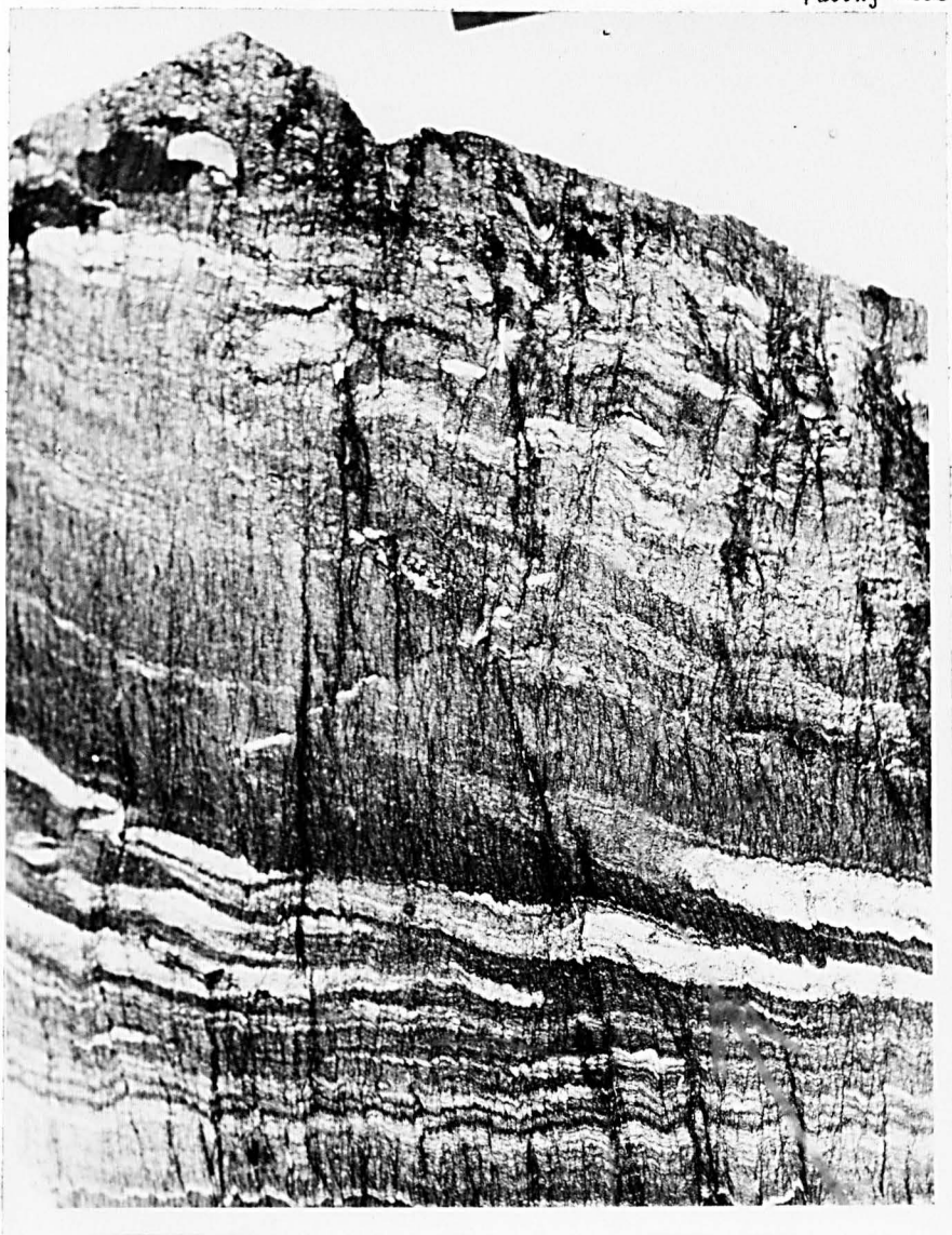
Actual size: 3.6cm by 2cm Top contact of breccia with undisturbed strata. Enlargement of slide (I495) of specimen obtained in Sulby Glen.
