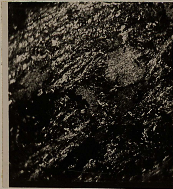
Magnification by 18. Crossed nicols. Slide I361, specimen from upper reaches Glen Auldyn, above fork near level on 6 inch map. Cordierite porphyroblasts showing pseudo-hexagonal form.
