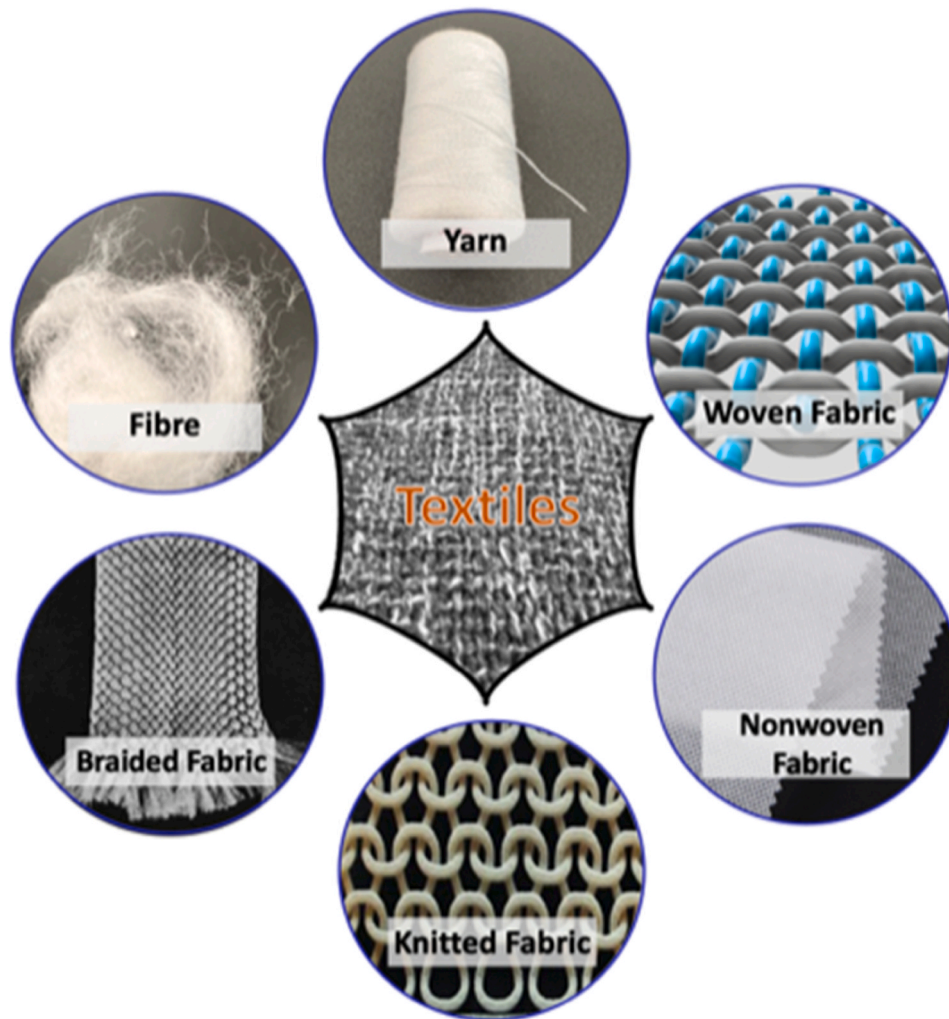
Fig. 5. Textile fibre [83], yarn [84], and various textile fabrics (braided [85], nonwoven [86], woven (self-drawn), knitted [87]).
