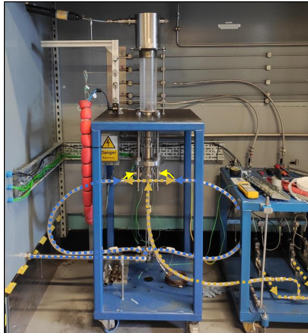
Figure 3.2.3-2 APGSB test rig during commissioning stage, indicating air (blue dotted line), fuel (brown dotted line) and mixture (yellow arrows) delivery paths.
