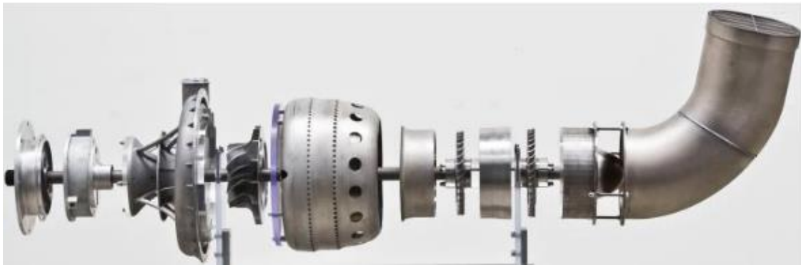
Figure 2.5.1-1 AM jet engine from Monash University and SAFRAN. Source: [191].
