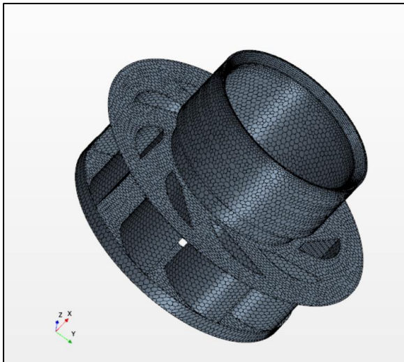
Figure 5.2-4 Surface mesh representation of swirler
