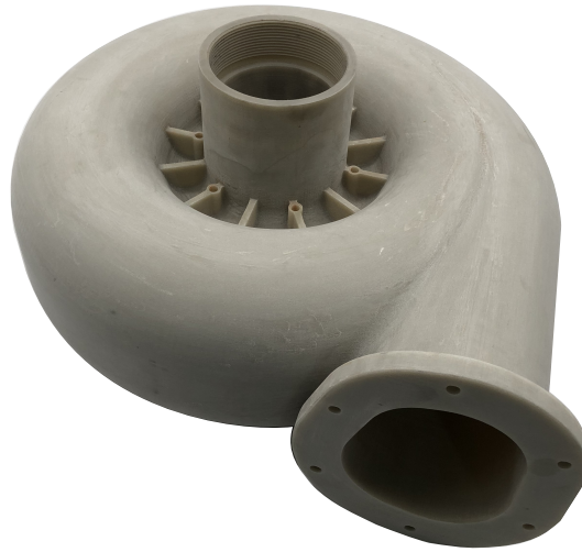
Figure 5.15: Front view of the manufactured volute
