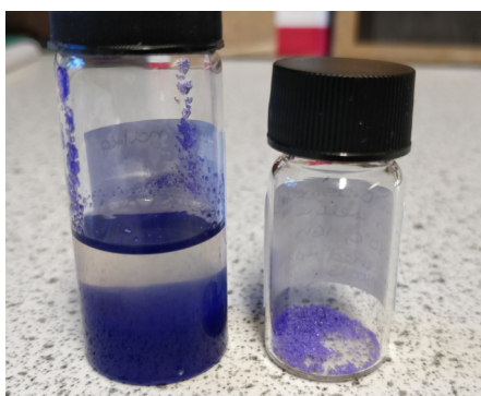
Figure 3.8: Post-reaction appearance of nickel(II) nitrate hexahydrate reacted in reline-0w at 150 °C, 10 h (left) and the solid isolated from the mixture by ethanol addition (right).
