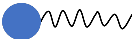
Figure 4.1: A representation of a typical surfactant molecule, showing the hydrophilic head region (blue) and the hydrophobic tail (black).
