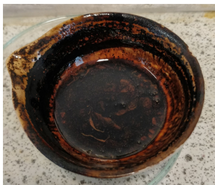
Figure 4.22: A image of the mixture obtained from the direct calcination of a solution of \text{ZnCl}_2 in \text{C}_{16}\text{TAB}/\text{DES} (urea:glycerol = 1.5:0.5) at 450 °C, 4h.
