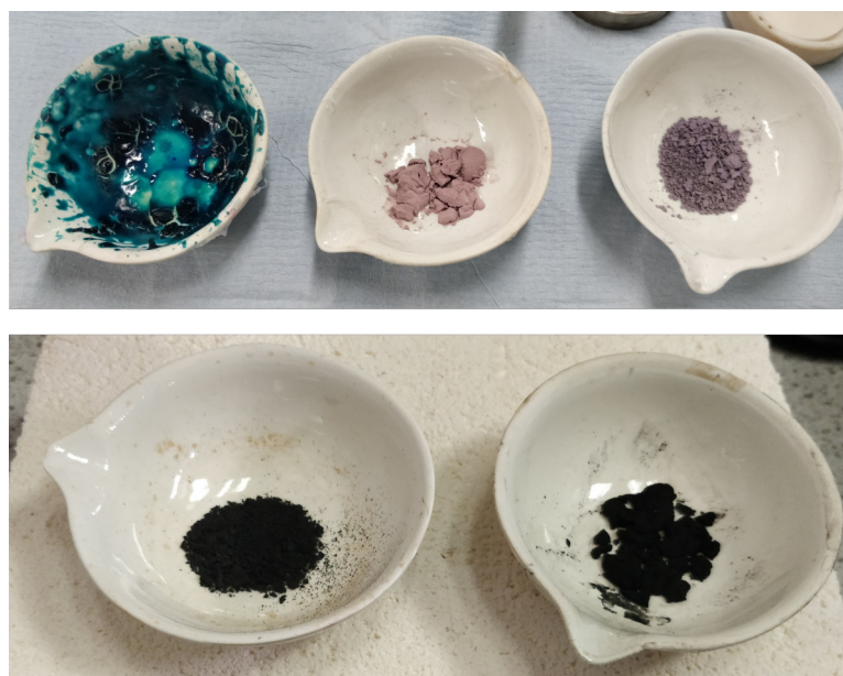
Figure 3.4: The appearance of the dried reaction mixture from cobalt(II) nitrate hexahydrate reacted in reline-0w, together with \text{CoCO}_3 synthesised in reline-2w and reline-10w. Black cobalt oxide powder formed following calcination at 300\text{ }^\circ\text{C} , 30 min of the products from the reline-2w and reline-10w reactions (bottom).
