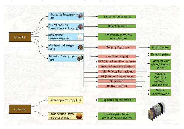
Figure 5: Overview of Infrared technologies for different investigations and Data Acquisition in Cultural Heritage. © Adapted from chsopensource.org
