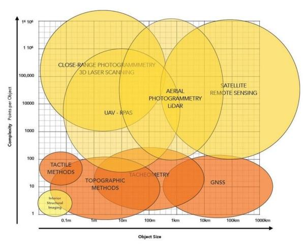
Figure 3: Survey techniques defined by object complexity (points captured) and size. © Adapted from Boehler & Heinz (1999) [71]. © UNESCO Chair on Digital Cultural Heritage at CUT.
