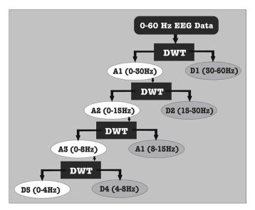
Fig. 4. Decomposition of EEG data in four levels.
